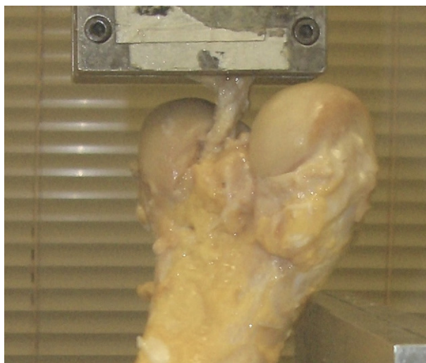
FIGURE 4. MTS setup for testing load to failure. The line of pull was directed in line with the graft and interference screw fixation to create the “worst-case scenario” of direct failure, oblique to lateral condyle and approximately 45° to the shaft.
