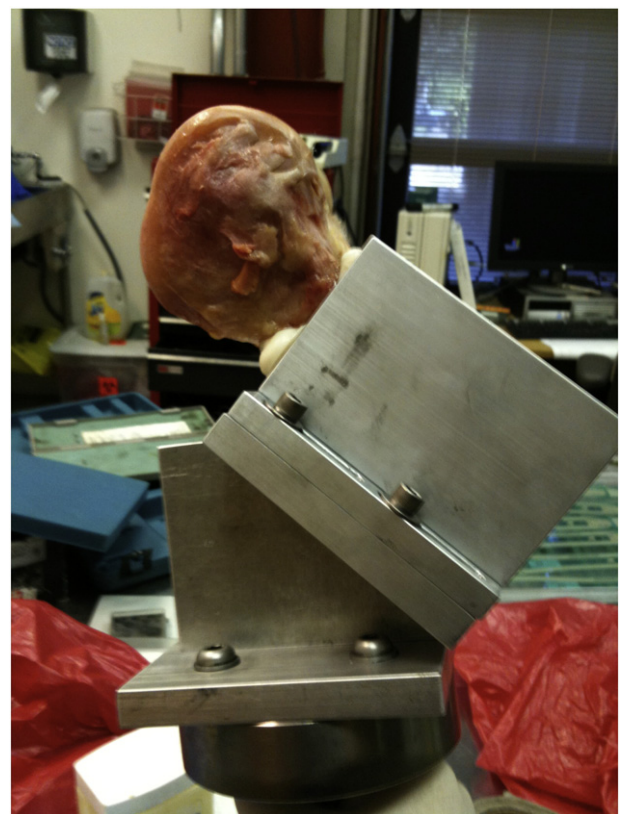
Fig. 1. Side profile of the MTS test fixture with a potted specimen inside. The square cylinder can slide up and down the 45^{\circ} incline, changing its height or depth.
